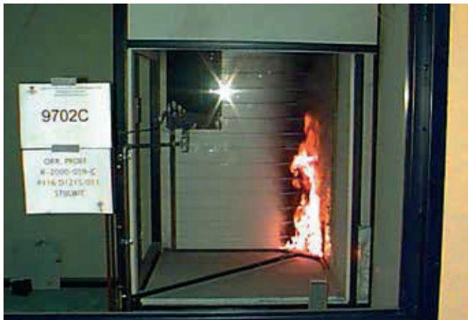
SBI - reaction to fire test
